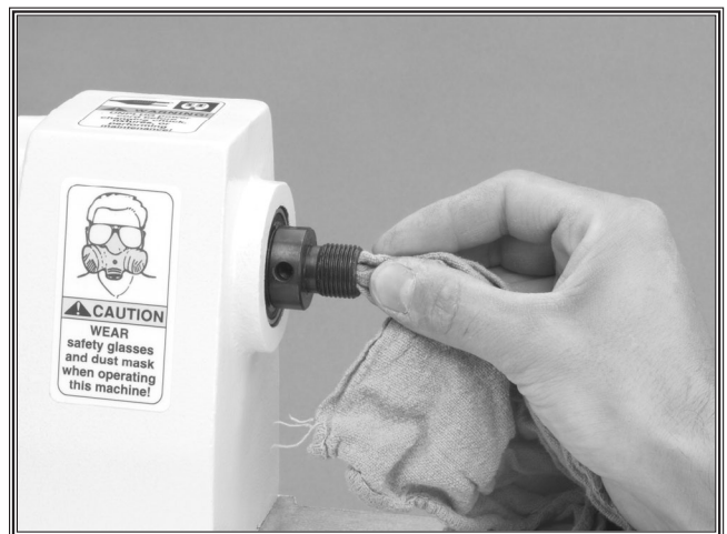
Figure 32. Cleaning spindle tapers.
